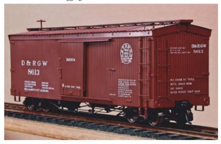
This boxcar in pristine condition is an early Accucraft import when they were made in 1:24 scale. Later Accucraft scaled its cars at 1:22.5 and the current 1:20.3 to reflect 3' gauge on the 45mm track. Darryl detailed the car for #8613 and rebuilt the trucks to the correct gauge for ½" scale. This makes this car both unique and rare.
