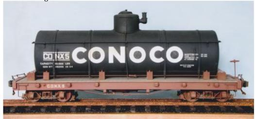
Conoco #5 is completely scratchbuilt and was started in 1983 until other priorities interrupted the progress of construction. In 2009, Darryl finally completed the model. Made from brass, almost every part is scratchbuilt including the trucks. Of course, the car features complete underbody detail and brake system. The prototype could be found on the Rio Grande and Rio Grande Southern as a part of a small fleet of Conoco tank cars operated on those railroads.
