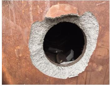
You could also see inside the cylinder at the front where the piston created the hole, and you could see pieces of the piston inside the cylinder cavity. In discussions with the train crew, it was determined that the piston had not completely broken, so it was not possible to simply slide the piston out. This meant that the entire assembly would have to be further taken apart prior to moving the locomotive and the train.
